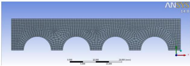
Fig.3. Meshed model of four tube bank
