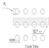
Fig. 1. Schematic diagram of a tube bank as a 2D model of compact heat exchanger with circular tube geometry.
